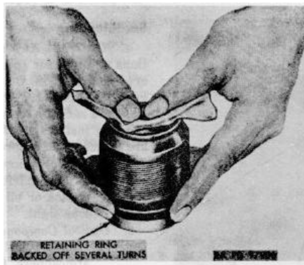
Figure 13. Applying pressure to loosen sealed lens.
